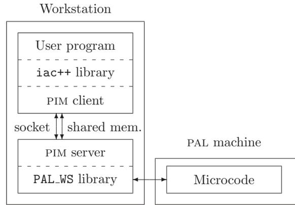
**Figure 2.** The user’s program uses the PIM client through the `iac++` library to talk to the PIM server. The server in turn uses the `PAL_WS` library to communicate with the PAL device.
