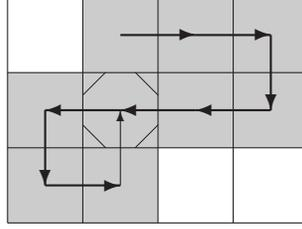
**Figure 8.** This convolution path involves nine shift operations, eight for calculations and one for returning to the origin.
