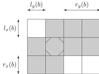
**Figure 5.** The functions  $l_d$  and  $r_d$  denote the extent of a template's bounding box on either side of its origin.
